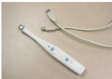
With an intraoral camera no larger than a toothbrush, images of a patient’s mouth can be gathered in a community setting and transferred to a dentist’s office for evaluation.
